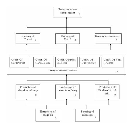
*Figure 4.4: System boundaries for scenario 2 (21 % biofuel supplements conventional fuel for the transport sector of Denmark)*
